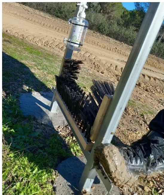
Figure 10: Footwear cleaning stations designed for the FAGESOS project. The stations included lateral brushes, lateral plates for removing excessive mud, and a disinfectant dispenser.
