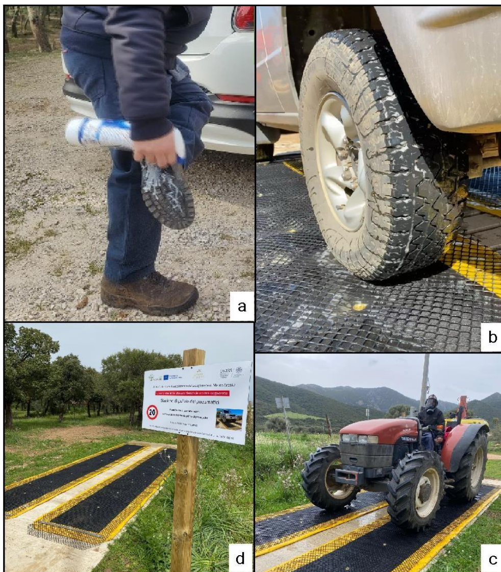
Figura 13. Mobile cleaning kits (a), Vehicles cleaning stations (b and c), signposting (d).
